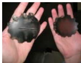
Above: Riser Feed Nozzles
