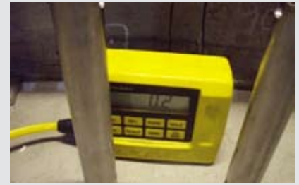
Photo - View of the Electronic Water Level used for checking Levelness of installed items
