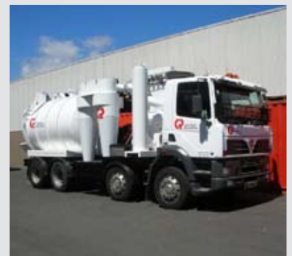
Photo - CR Wet/Dry Vacuum Truck with Dresser Roots Blower (76m 3 /min) and 9500L Tank
