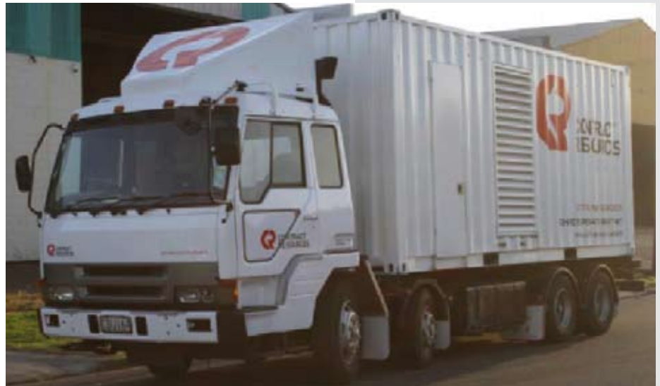
Photo - Containerised 265HP Pump
