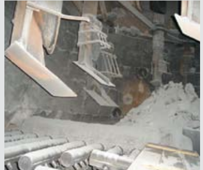
Photo - Coke build up on the grates
