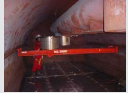
Photo - Purpose build gantry crane
