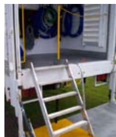
HP044 - Rear step and tail lift into workshop area
