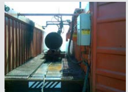
Photo - The fully integrated automated exchanger cleaning unit in action
